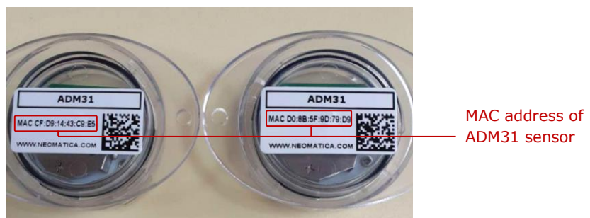
Figure 2 — Identifying the MAC-address of ADM31 sensor
