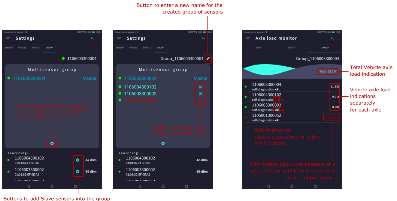
a) creation of a group of sensors for monitoring axle load indications
