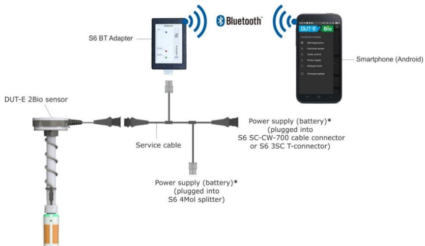
Figure 38 – Connection diagram for wireless setup of DUT-E CAN/DUT-E GSM/DUT-E 2Bio fuel level sensor
