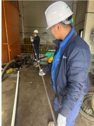
DUT-E sensor extension up to 8 meters
