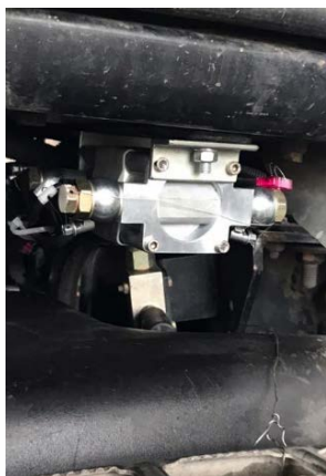
DFM 500D fuel flowmeter, installed on the tractor
