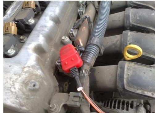
Figure 20 — Examples of Crocodile connection
