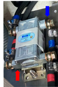
Left: DFM D S7 flow meter connected to the supply (→) and return (←) fuel lines Right: Fuel consumption data displayed on the Raymarine HybridTouch screen
