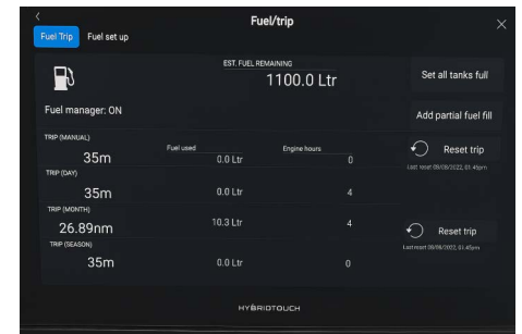
Left: DFM D S7 flow meter connected to the supply (→) and return (←) fuel lines Right: Fuel consumption data displayed on the Raymarine HybridTouch screen
