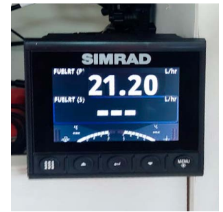
Fuel consumption displayed on Simrad IS42J
