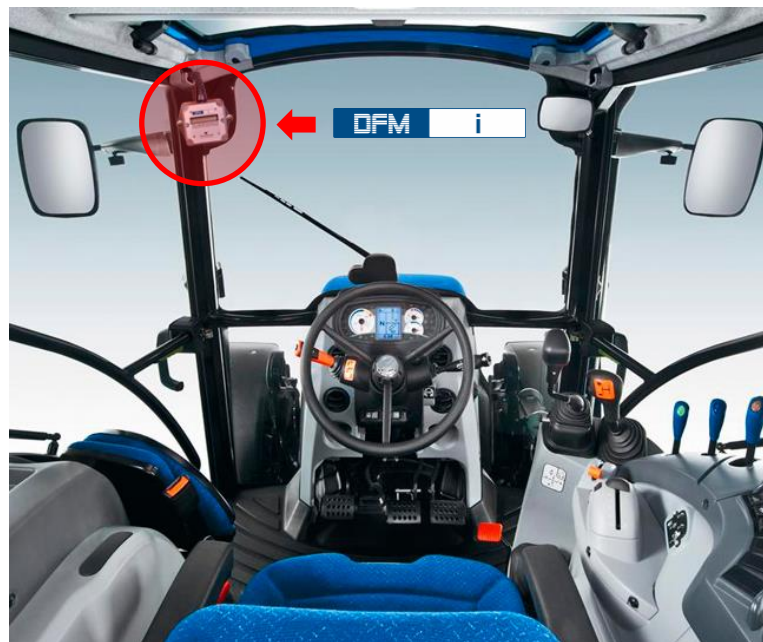
Figure 11 — Example of DFM i mounting location in the tractor driver's cabin
