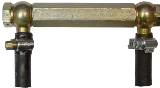
Figure 3 — Connector fitting for temporary mounting into the fuel system, instead of DFM fuel flow meter
