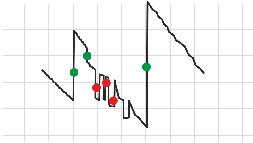
Unfiltered signal – true (●), and false (●) fuel fill-up and draining events are visible
