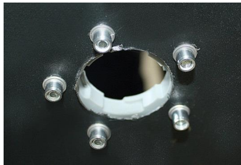
b) installed fastening plate view of from inside of tank
