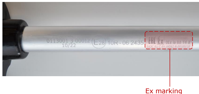
Figure C.1 – Placing of Ex mark on DUT-E S7
