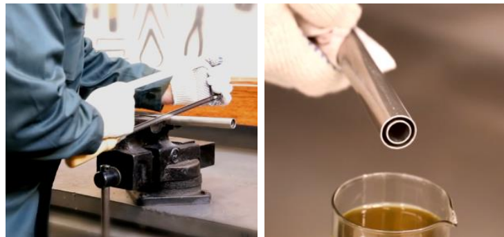
Figure 19 — Measuring probe cutting and flushing the cut with fuel
