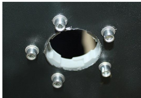
b) installed fastening plate view of from inside of tank
