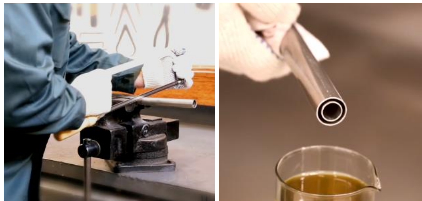
Figure 14 — DUT-E AF measuring probe cutting and flushing the cut with fuel
