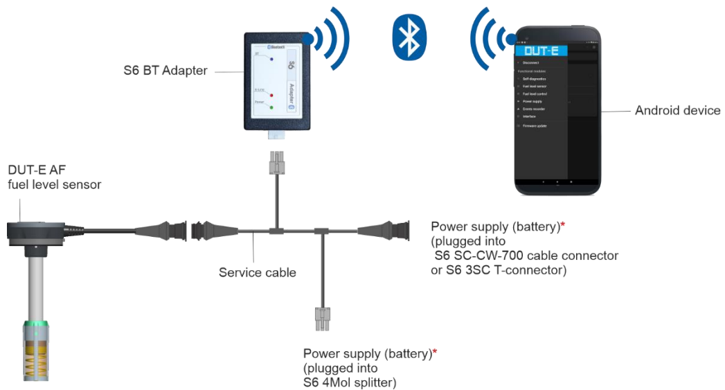
Figure 24 — Scheme of wireless connection of DUT-E AF to Android-based device using S6 BT Adapter
