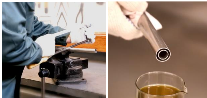
Figure 14 — DUT-E CAN measuring probe cutting and flushing the cut with fuel
