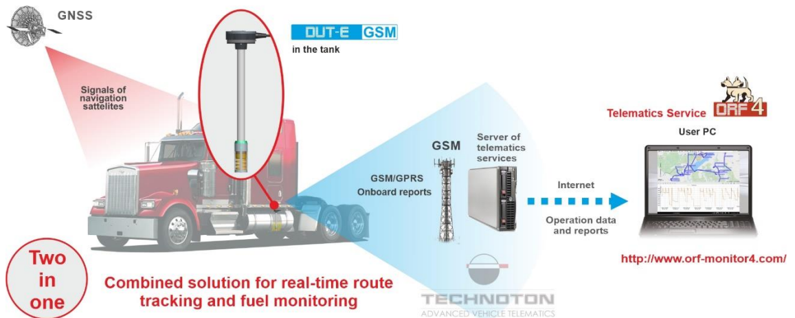
Figure 3 — Example of DUT-E GSM operation as part of the Telematic system
