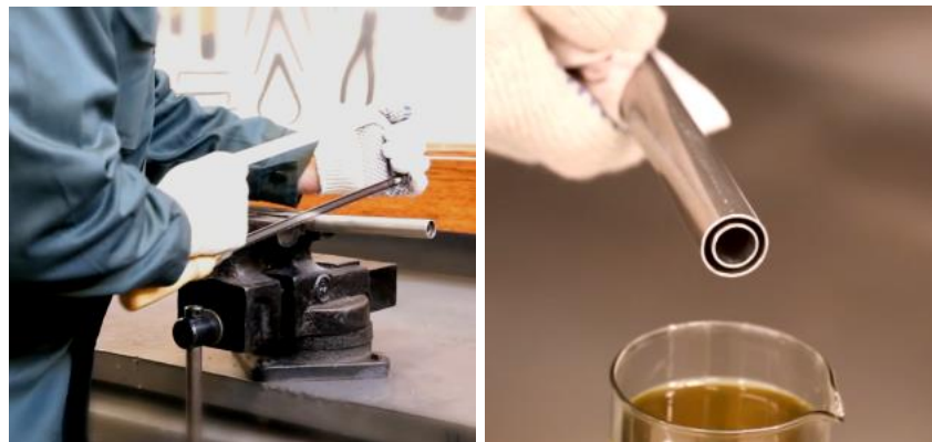
Figure 16 – DUT-E GSM measuring probe cutting and flushing the cut with fuel
