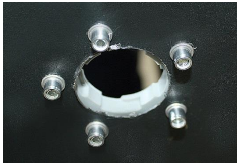
a) threaded rivets procedure of installation
