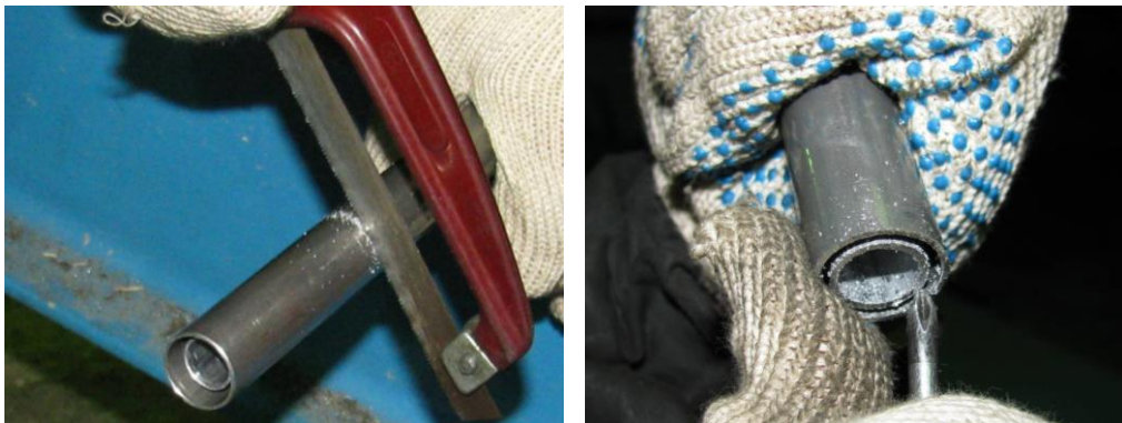
Figure 3 — Cutting a sensor and removal of barbs after cutting
