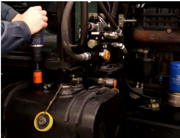
Figure 2 — Drilling a tank according to the drawing with the holes' locations indication
