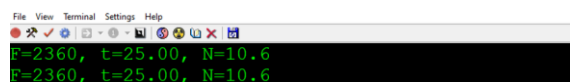
Figure F.2 — Example of display of parameters transferred by DUT-E 232 with the set period of data transfer, according to ASCII text protocol, in the software that registers data of COM-port
