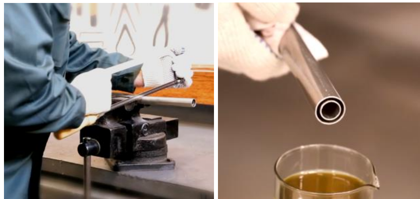
Figure 14 — DUT-E measuring probe cutting and flushing the cut with fuel
