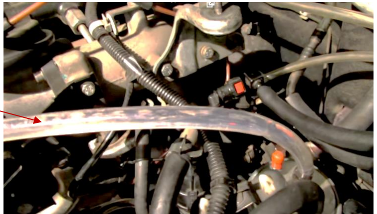
Figure 5 — Visual detection of air content in the fuel
