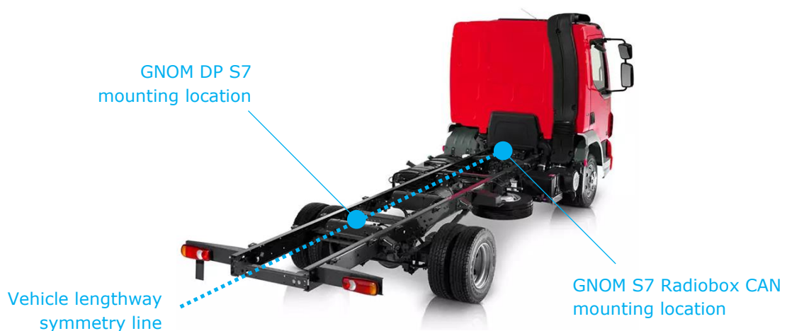
Figure 7 — Example of choosing a location for mounting GNOM S7 Radiobox CAN converter for reception of a signal from GNOM DP S7 wireless sensor
