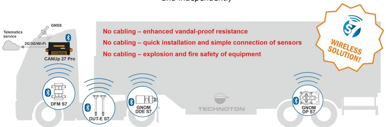
b) example of axle load monitoring during the comprehensive monitoring of the vehicle performance parameters by means of S7 Technology
