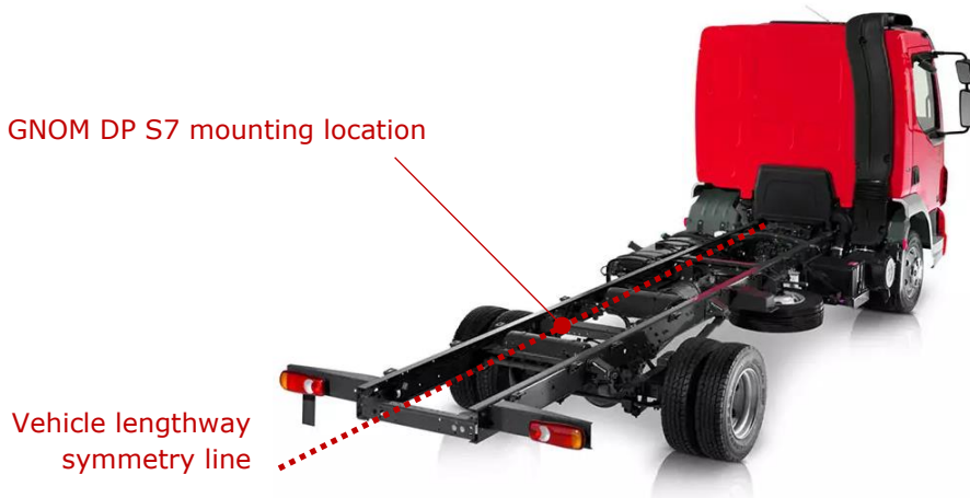
Figure 18 — Selection for GNOM DP S7 mounting location for monitoring the Vehicle axle load
