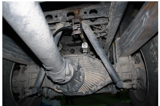
a) elastic element is mounted in the same plane as the pivoted lever of the sensor
