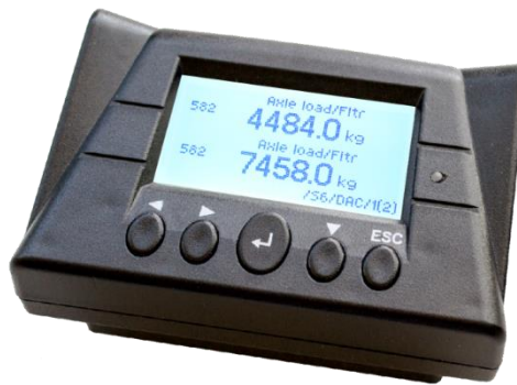
Figure 40 — MasterCAN Display 35 G exterior view
