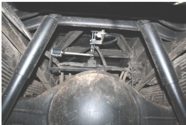
b) elastic element is perpendicular to the pivoted lever of the sensor
