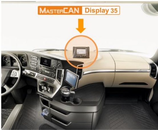
a) place of installation
