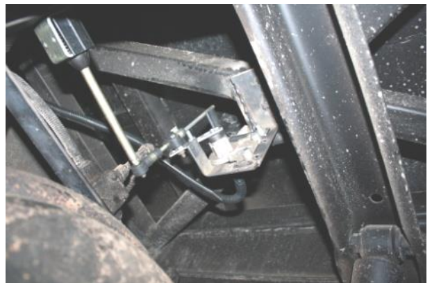
b) elastic element is perpendicular to the pivoted lever of the sensor
