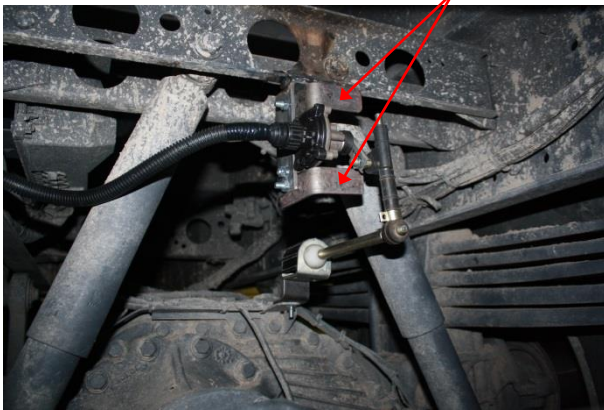
a) elastic element is mounted in the same plane as the pivoted lever of the sensor
