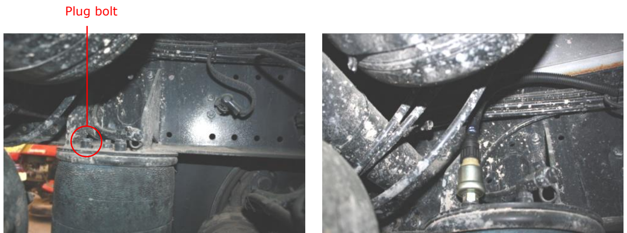
Figure 26 — GNOM DDE mounted into suspension air balloon
