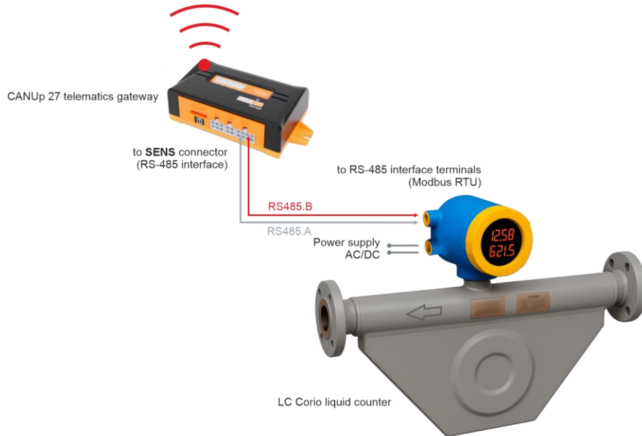
a) connecting LC Corio via the RS-485 interface to the CANUp 27 Genset telematics gateway
