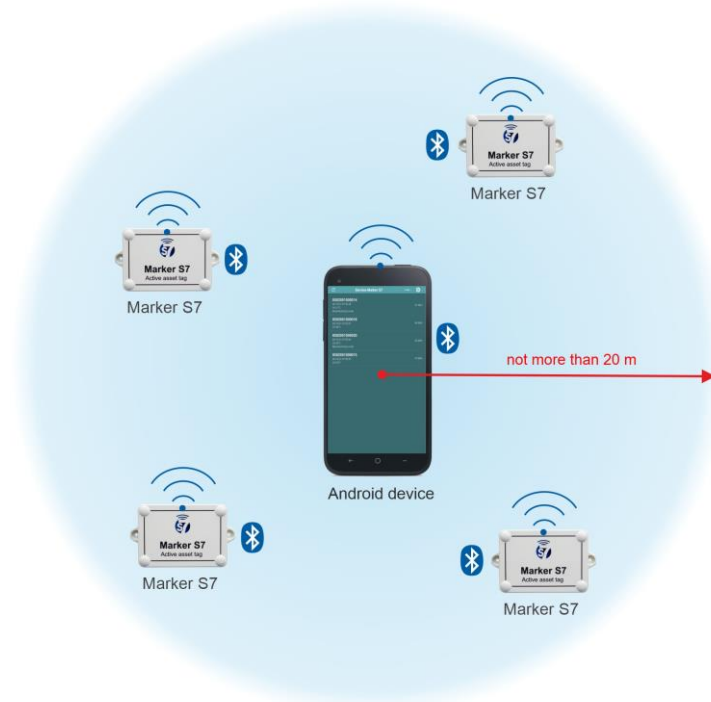
Figure 9 — Testing the Marker S7 tags operation by means of S7 Technology using the Android-based device
