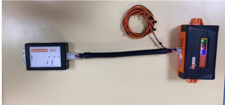
Figure 3 — Using S6 027 cable to connect Units via S6 Technology and power the system
