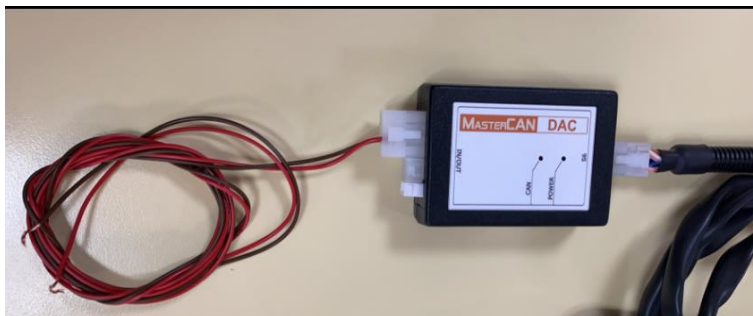
Figure 5 — Connecting assembled connector to the discrete output of MasterCAN DAC 15
