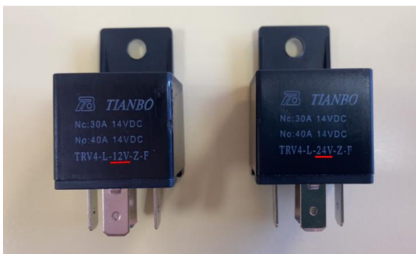
Figure 7 – An example of finding out supply voltage of the coil when selecting a relay and installing a relay in a connector
