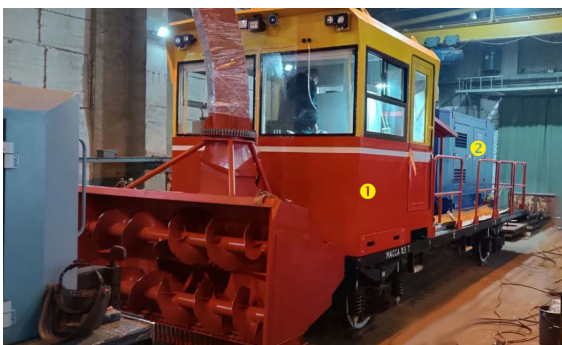
Auger-rotor snowplow in the production facility ① operator's cabin, ② diesel generator unit
