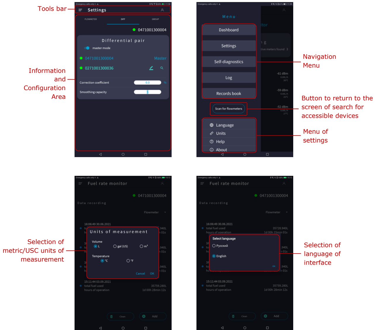
Figure 3 — Interface of Fuel Rate Monitor mobile application
