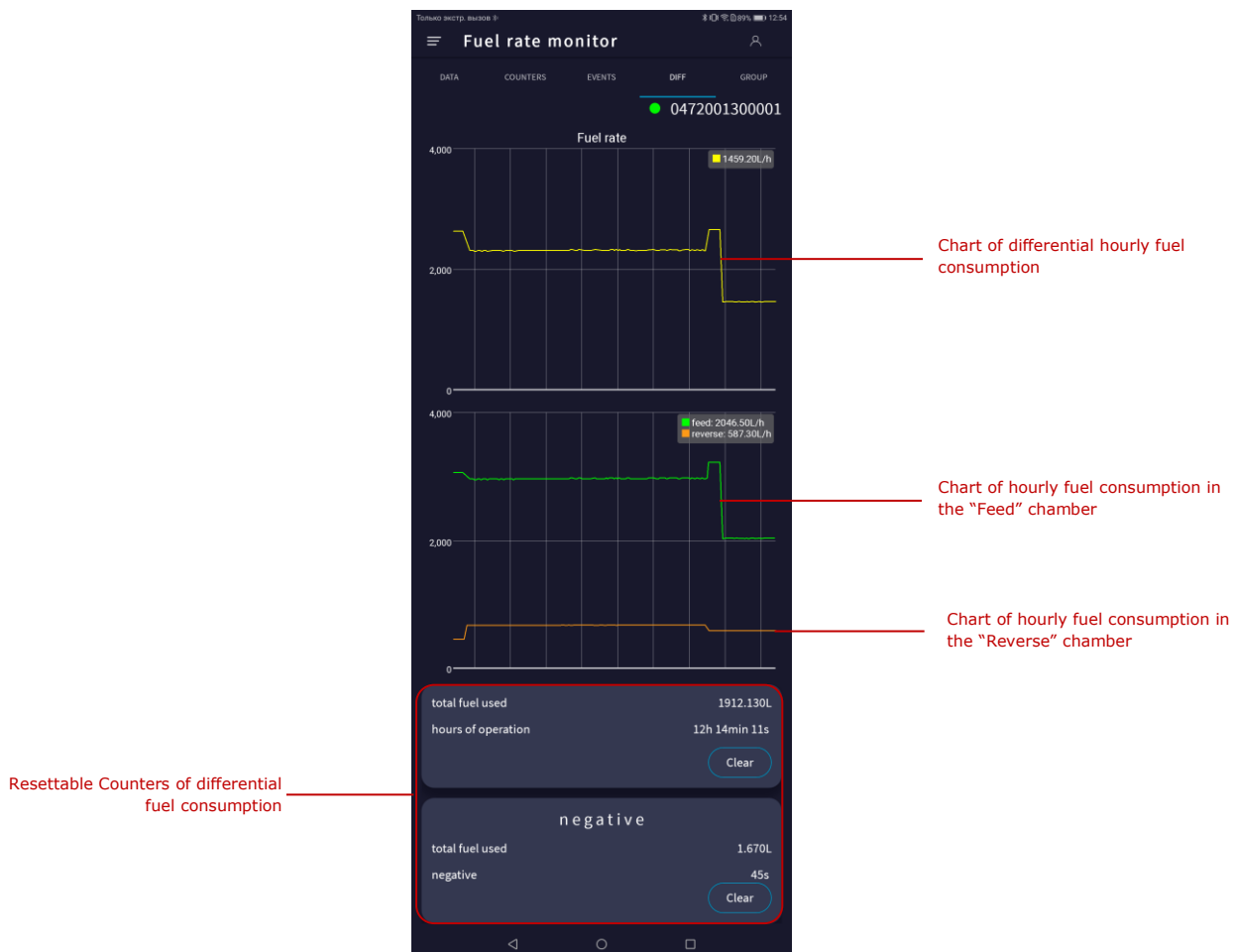
Figure 8 — Example of real time display of development curves of hourly fuel consumption and of Counters for the operating differential pair of flow meters
