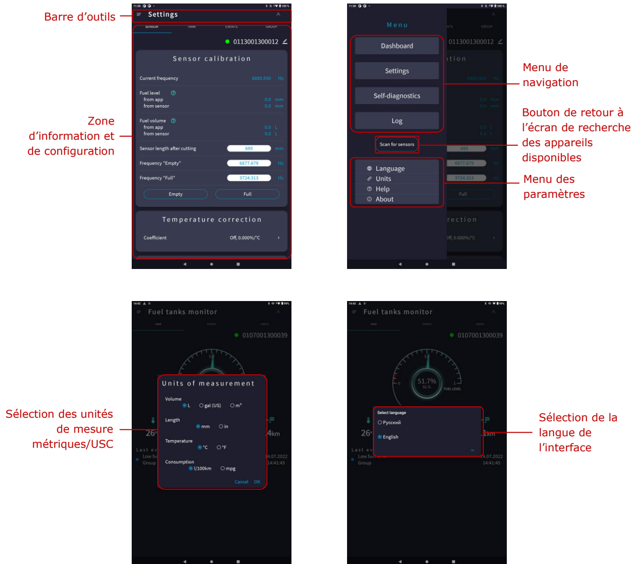
Figure 16 — Interface de l'application mobile Fuel Tanks Monitor
