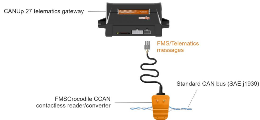
Figure 24 — Safe integration of Automotive CANbus into Telematics system using FMSCrocodile CCAN
