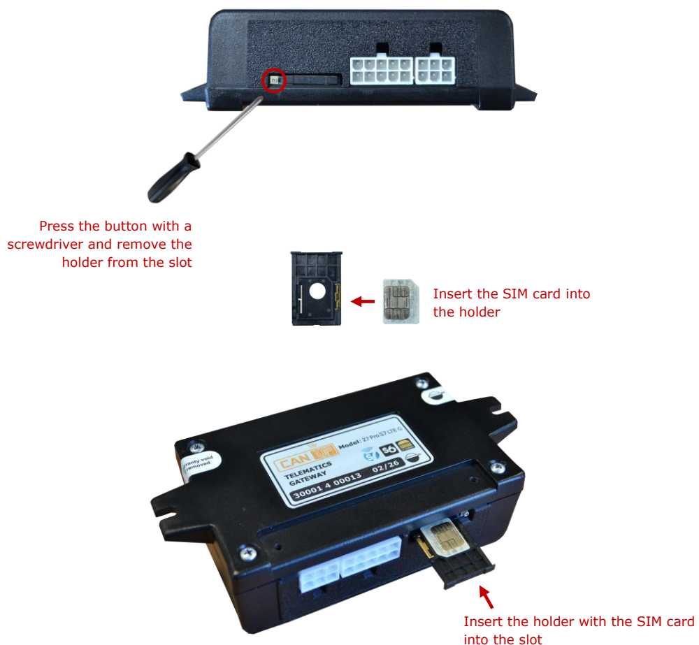
Figure 11 — SIM card installation in CANUp 27
